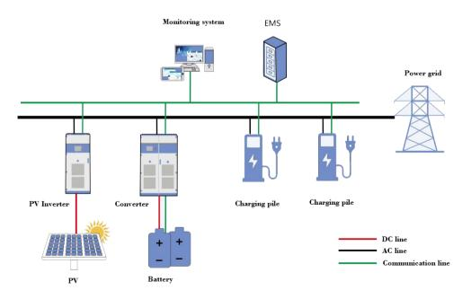
Some remote areas without power need to build their own power grid due to sparse population and far distance from the main grid. Photovoltaic energy storage and micro-grid technologies can be adopted to realize system power supply. Different circuit topologies can be adopted according to different power requirements to meet different customer needs.
